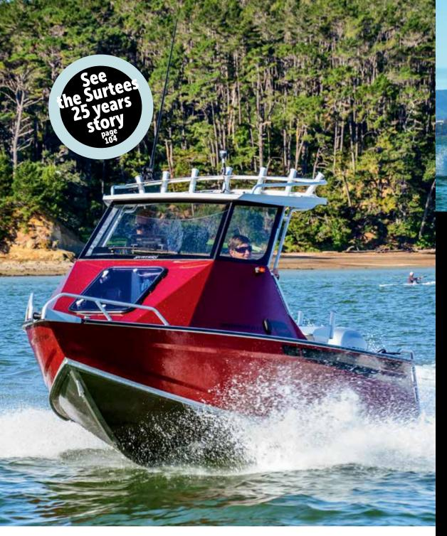
at the most efficient speed of 20 knots she was using just over 11 litres per hour. This gives an effective range of around 150 nautical miles, well beyond the limits of most day trips.
